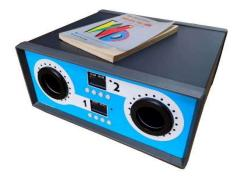
The BL672 is a benchtop blackbody calibration source utilizing a digital indicating temperature ambient 30°C to 50°C (86F to 122F). Two 60mm diameter end closed tube is heated or cooled with an internal solid state thermoelectric heat pump. It has a built-in digital temperature controller to provide accurate, stable temperature as well as to provide readout.
